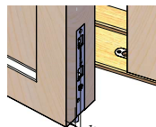
Image 1: Measured 12mm from the front to the center of the bolt for placement of the strik.
