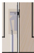
Image 3: Guide fitted at the bottom as well as glider on active door leaf centralized on the latch bolt.
